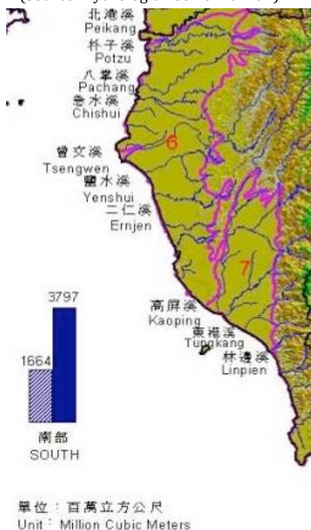
Figure 10. The pumped and recharged of ground-water in south Taiwan in 1936. (Source: Hydrologic Book of Taiwan)
